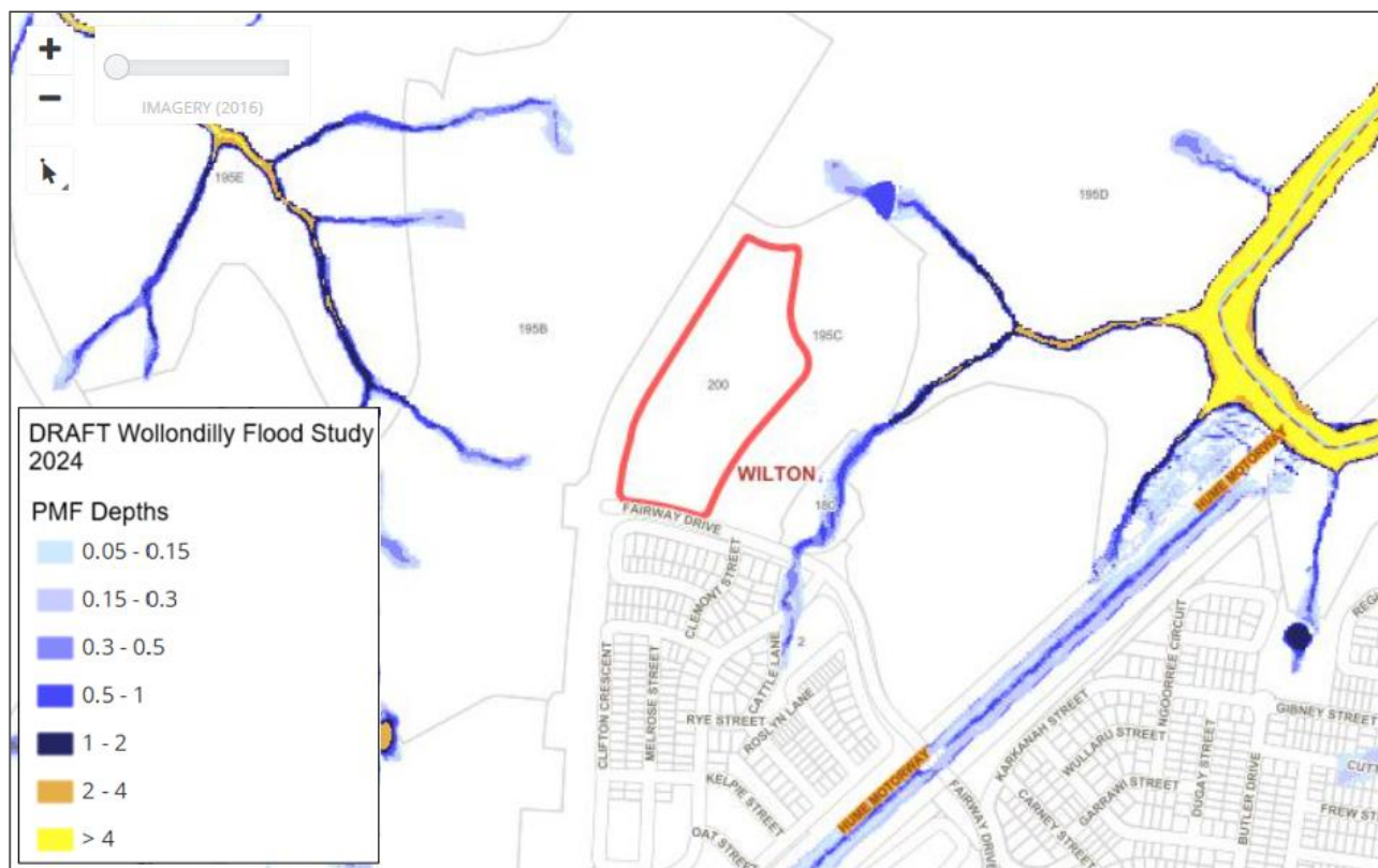
Figure 12: Peak flood depth in the Wilton area during the PMF event. Source: adapted from Wollondilly City Council, 2024.
